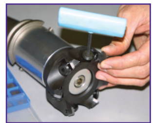
Installing Carbide Inserts (left-handed thread)
