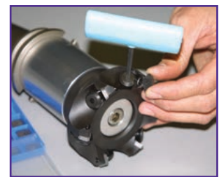
Installing Carbide Inserts (left-handed thread)
